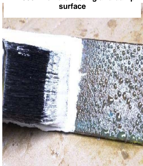
RL 500PF on a sweating and damp surface
