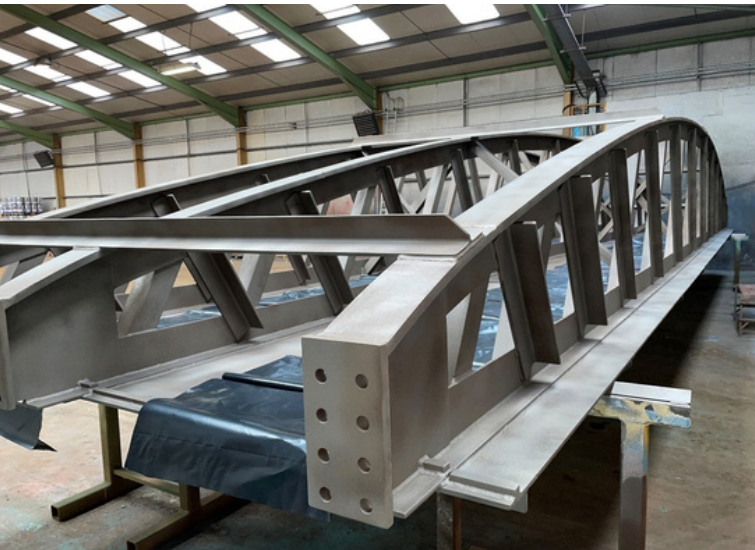
After Surface Preparation
