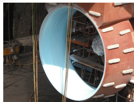
RA 500CG applied to Kort Nozzle
