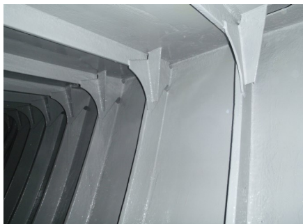
Sea Water Ballast Tanks: RS 500P & RA 500M
