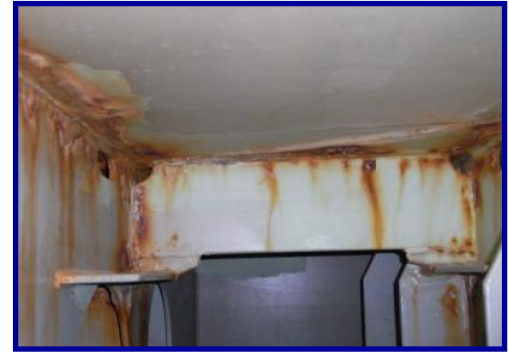
Double-bottom tanktop after 7 years in-service
