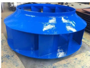
View of impeller completion
